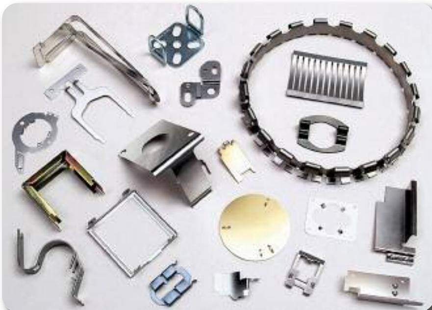
These parts all resulted from the fourslide process as performed at Fourslide Spring and Stamping, Bristol, CT. The process boasts production rates to 15,000 pieces/hr., depending on part size and complexity. Fourslide production can dramatically decrease tooling costs and lead time compared to traditional stamping in certain applications, and since the process typically starts with material the width of the finished part, it generates minimal scrap.
